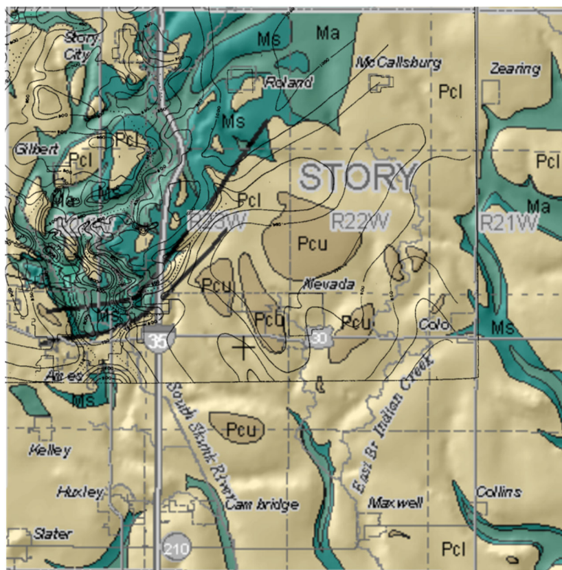
Figure 2. The surface topography of the bedrock underneath the glacial drift in Story County. The contour lines are in 50 foot intervals. (Kent & Sendlein, 1972; Witzke, et. al. 2014).
