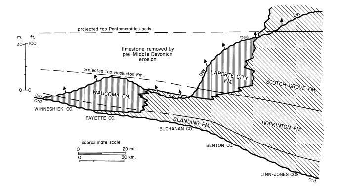
Figure 2. Stratigraphic cross section showing the positions of limestones in the Waucoma and LaPorte City formations, and their stratigraphic relationships to dolomitized Silurian sequences in Iowa.
