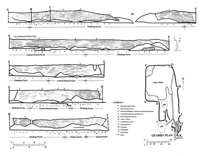
Figure 4. Bedding within carbonate mounds of the Johns Creek Quarry Member as seen along the walls of the Manternach Quarry, Jones County (Stop 2). Traced from photo mosaic; no vertical exaggeration. White areas show where walls are covered by talus or quarry piles. General extent of central mound and flanking facies is delineated.
