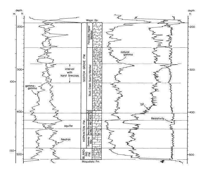
Figure 2. Stratigraphic section from Robins corehole, Linn County, shown with a suite of geophysical logs (modified from Wahl and Bunker, 1986; Witzke, 1991, pers. comm.)
