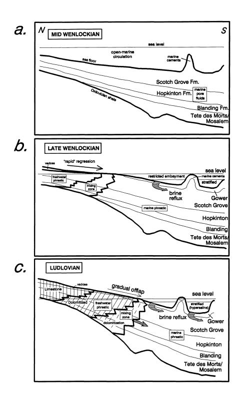
Figure 3. Schematic drawing of Wenlockian to Ludlovian depositional, hydrologic, and diagenetic events in the Silurian sequence of Iowa. Limestones at the perimeter of the East-Central Iowa Basin were rapidly flushed of marine pore fluids, and were diagenetically altered by meteoric phreatic fluids. Subsequent gradual basinward migration of the marine-meteoric mixing zone may have led to the pervasive dolomitization of the remaining sequence.
