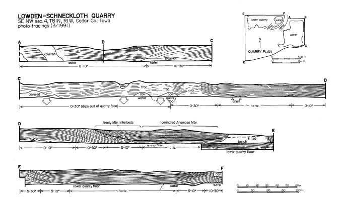
Figure 12. Carbonate mound facies of the Scotch Grove and Gower formations exposed at the Lowden-Schneckloth Quarry, Cedar County (Loc. SNQ, Fig. 1). Figure displays bedding as seen along quarry walls, traced from photo mosaic. General dips are noted (arrows show where beds dip out of quarry face). No vertical exaggeration.
