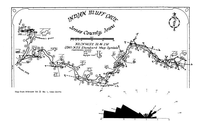
**Figure 1.** Map of Indian Bluff Cave (Hedges, 1974), with cave fractures shown as solid lines, and prominent surface fracture trends (illustrated by the rose diagram), which control passage trends shown as dashed lines.
