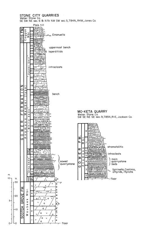
**Figure 8.** Graphic stratigraphic section of exposed interval seen in the Stone City quarries (Stop 4). Unit descriptions are provided in text. Mo-Keta quarry section is provided for comparison. See page 86 for lithologic symbols.
