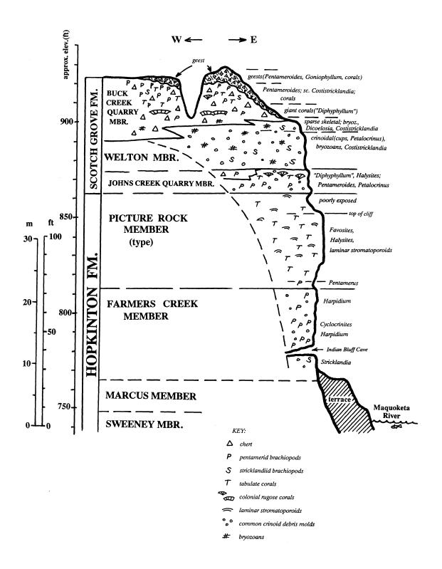
**Figure 3.** General stratigraphic section in the Picture Rock area, extending from county park (Block A, Fig. 1) on the east to the Hanken Quarry (Block C, Fig. 1) on the west.
