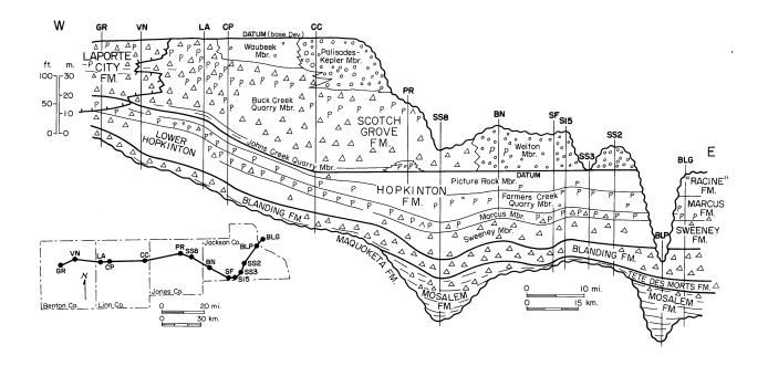
**Figure 6.** Stratigraphic cross-section of Silurian dolomite units, east-central Iowa. LaPorte City Formation is a western limestone facies. Control points include both core and outcrop sections. Datum shifts from base of Devonian in the west to base of Scotch Grove Formation in the eastern outcrop. See page 86 for lithologic symbols.
