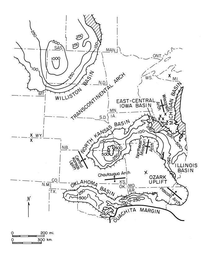
Figure 7. Generalized Silurian isopach map, Midcontinent area. Isopachs are in feet. Structural elements are labeled. Location of Silurian outliers marked by X. Silurian edge is hachured. Silurian outcrop areas are cross-ruled.
