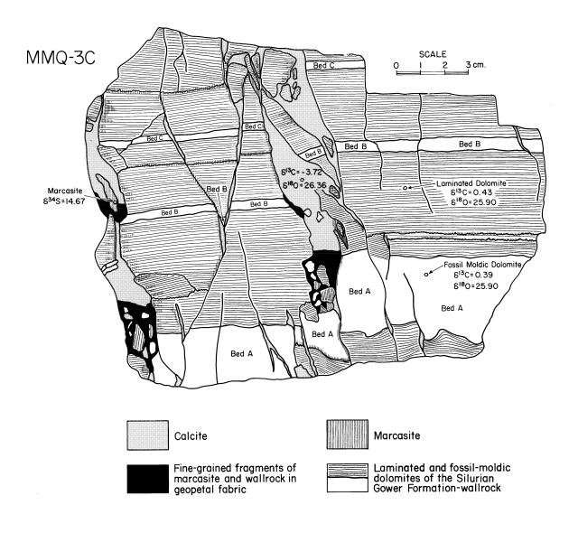
**Figure 4.** Drawing of polished slab surface of rock sample MMQ-3C (Gower Formation, Cedar Rapids Martin Marietta Quarry), showing microstructural detail of isotopic sampling sites. Note samples in laminated and fossil moldic dolostones. Oxygen isotopic data in this diagram were reported relative to the SMOW standard. From Garvin et al., 1987.
