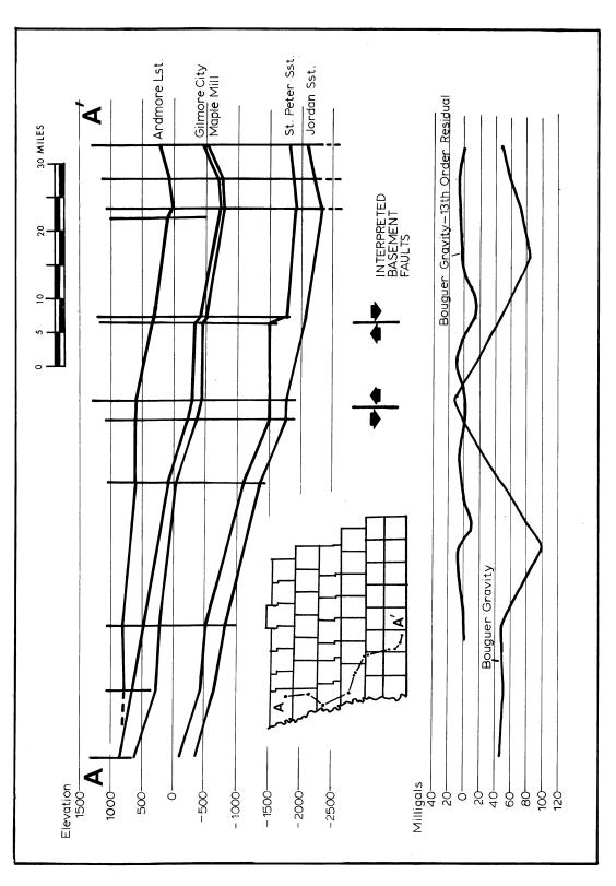
Structure section on NW-SE direction across the Thurman-Wilson structural zone showing the structure and corresponding gravity anomaly. Displacement in the lower Paleozoic is greater than displacement in the upper Paleozoic indicating continued tectonic activity along the zone. Figure 4.
