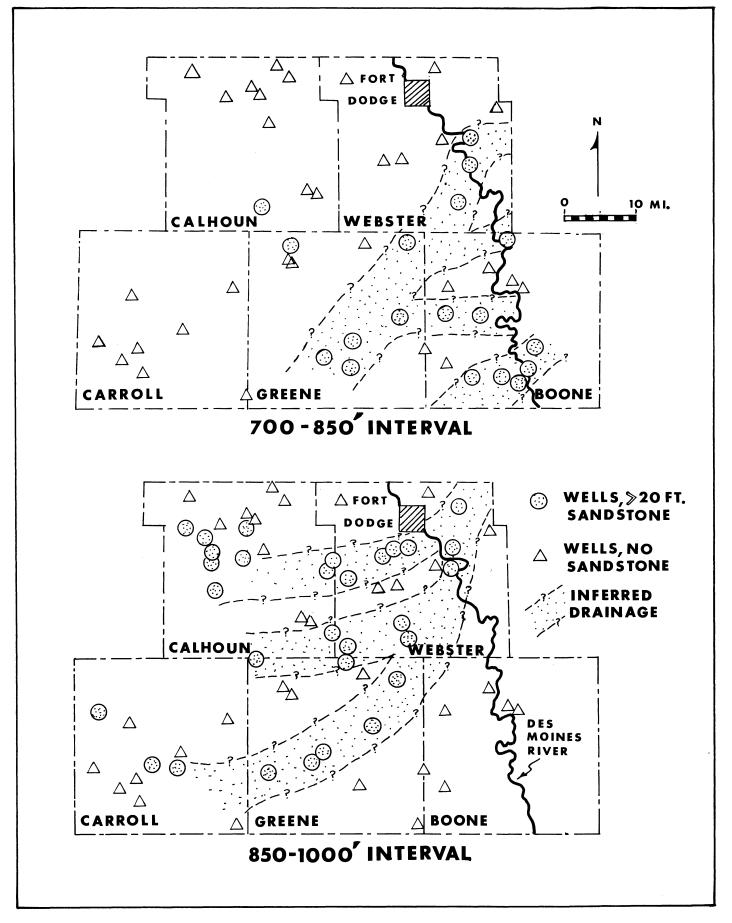
Figure 11. Maps showing the distribution of sand bodies in the subsurface in the area immediately southwest of the sandstone outcrops along the Des Moines River. The paleodrainage is inferred from well log data.
