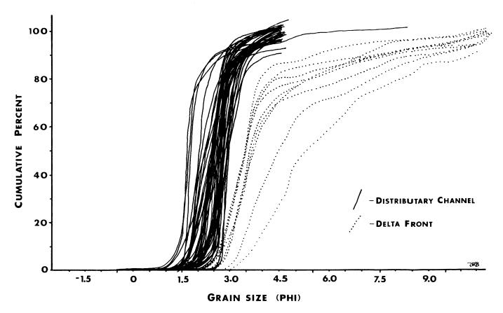
Figure 23. Cumulative weight percent (arithmetic) versus grain size (phi) for 46 samples of lower Cherokee Group samples.
