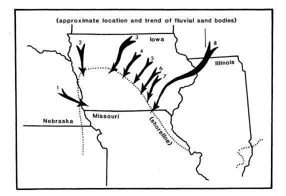
Figure 8. Inferred Cherokee paleodrainage based on outcrop and subsurface evidence of sand bodies. The sand bodies are at different stratigraphic levels within the Cherokee and are considered to be of different ages. (1) Nemaha ridge source, (2) source from the north, (3) Fort Dodge-Holiday Creek area, (4) Dolliver Park area, (5) Ledges area, (6) Altoona (subsurface) area, (7) Red Rock Dam area, (8) Southeast Iowa-northeast Missouri area.
