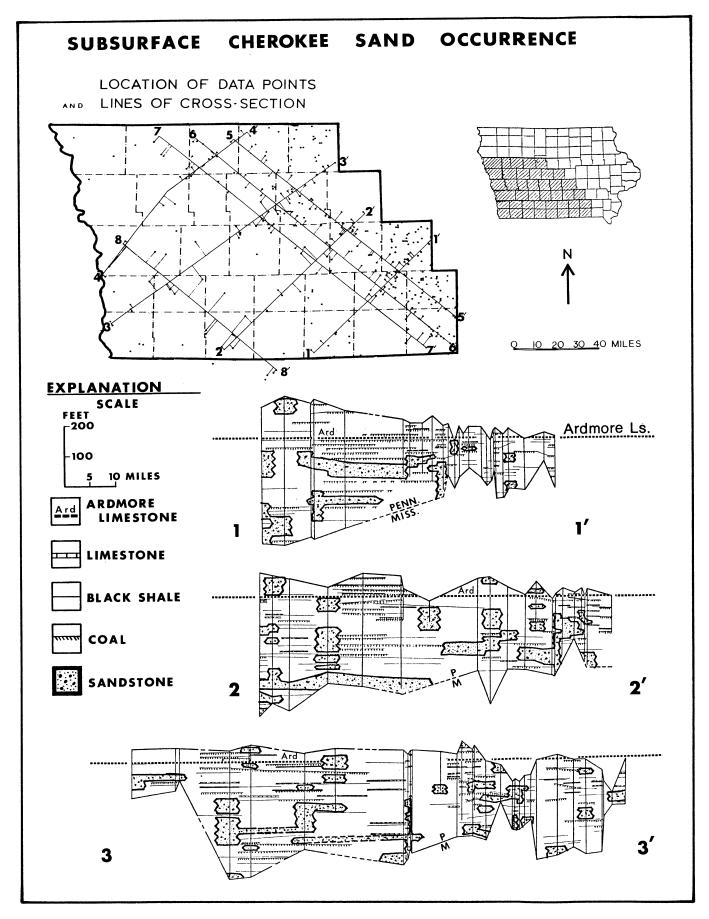
Figure 10. Index map showing well control and direction of cross-sections. 1.-8. Structure sections showing distribution and occurrence of sandstone bodies in the subsurface with reference to the Ardmore Limestone.
