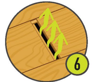
6 Gaps in suspended floors
