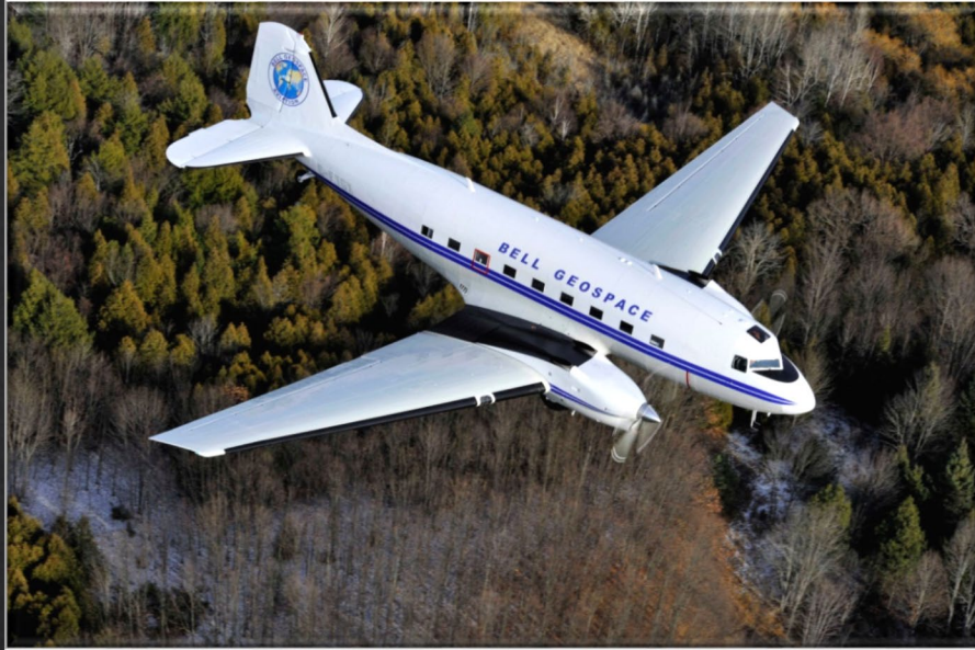
BT-67 fixed wing turboprop aircraft that carried the gravity survey instrument
