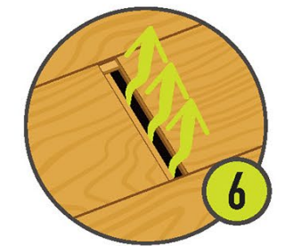
6 Gaps in suspended floors
