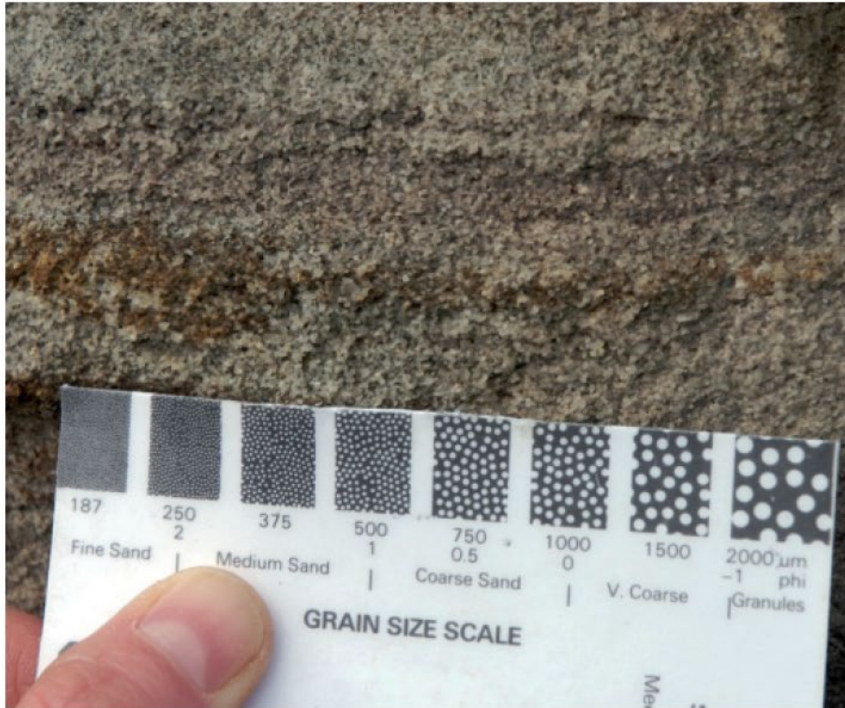
Figure 2.16 Use of a grain-size chart to determine the average grain size. (a) In this case the average grain size is 500 \mu\text{m} . The grain size varies between 375 and 750 \mu\text{m} . (b) Close up view of (a).
